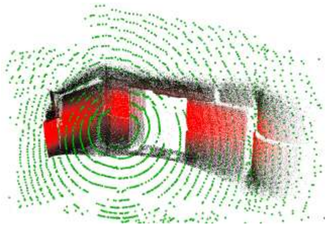
Figure 4: View of 3D Laser Data Point Cloud Aligned With 3D Sonar Point Cloud
